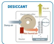
This model features a desiccant wheel instead of a rotary compressor, it will keep on dehumidifying at maximum capacity even below an ambient temperature of 15°C. Ideal for cellars, garages, caravans, boats, storage rooms. No compressor, no harmful refrigerant gas
