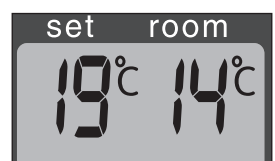
G: The required temperature on the left, the measured temperature on the right.
