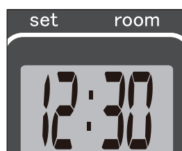
F: When the 4-digit stops blinking, the setting has been locked to the indicated value.
