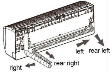
2. When select leading out the pipe from left or right, please cut off the corresponding hole on the bottom-case.
