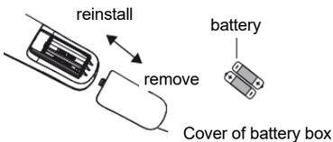
1. Press the back side of remote controlled marked with «
